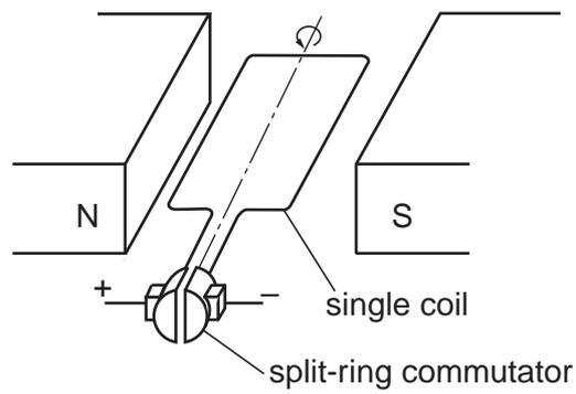
The split-ring commutator reverses the current in the coil as it rotates.
